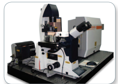
Catalyst-IRIS AFM- Raman system for biology and transparent samples. (Image courtesy of Aleksander Balter, Physics Department, UMK, Torun, Poland.)
