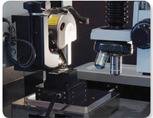
Dimension Icon-Raman in AFM measurement position. Here acquiring quantitative nanomechanical data on a polymer blend.
