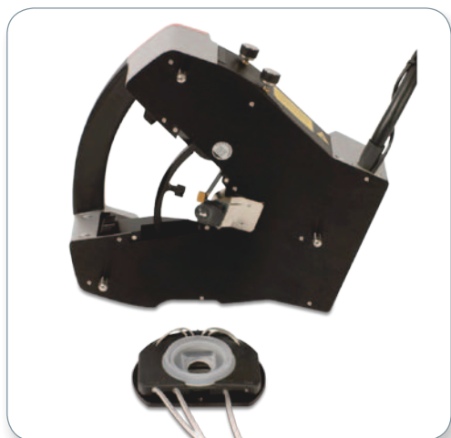
Catalyst head with perfusion accessory for long-term live cell studies.
