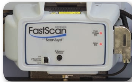
Scanner Resonant Frequency X-Y: 2.70kHz, Z: >50kHz.
