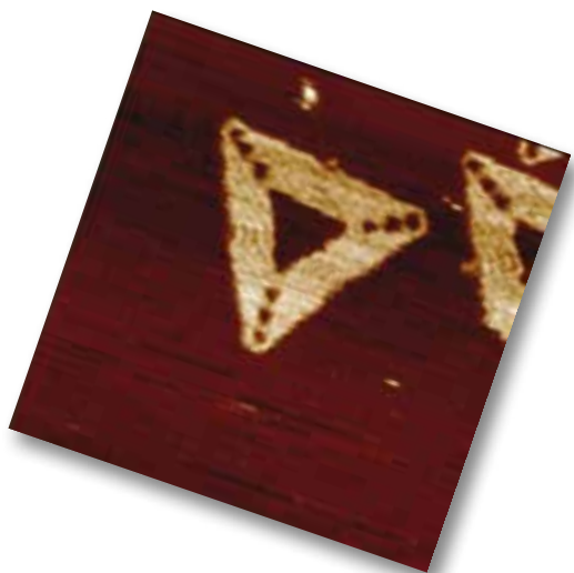
Individual triangular self-assemblies of origami-DNA on mica, imaged in liquid. Image size 250nm. Closed-loop. Revealing individual strands and fine structure at the connection points. (Sample courtesy of P. Rothmund, Caltech.)
