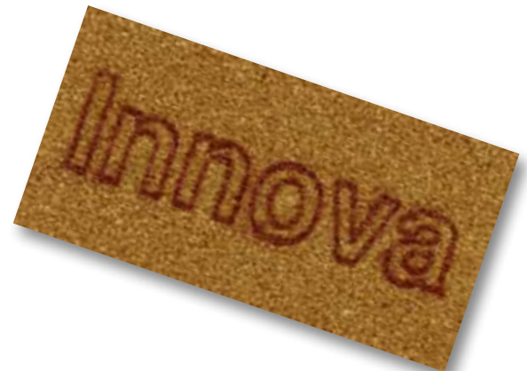
Piezoforce lithography on thin PZT film.
