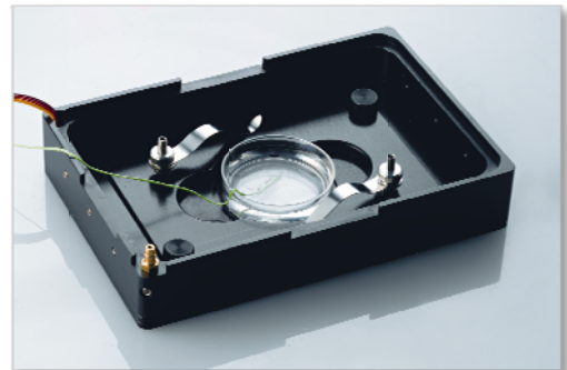
External T sensor in Petri, during Self Calibration
