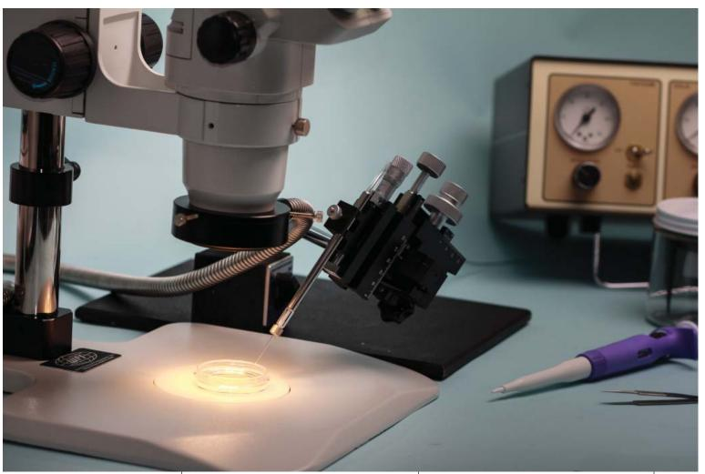
The basic Zebrafish Injection system includes: Nikon SMZ25 Microscope with stand, PV820 PicoPump, M3301 Micromanipulator, 5430-ALL PicoNozzle Kit, M10 Magnetic stand, Fiber Optic Illuminator, 5052 Steel base plate.
