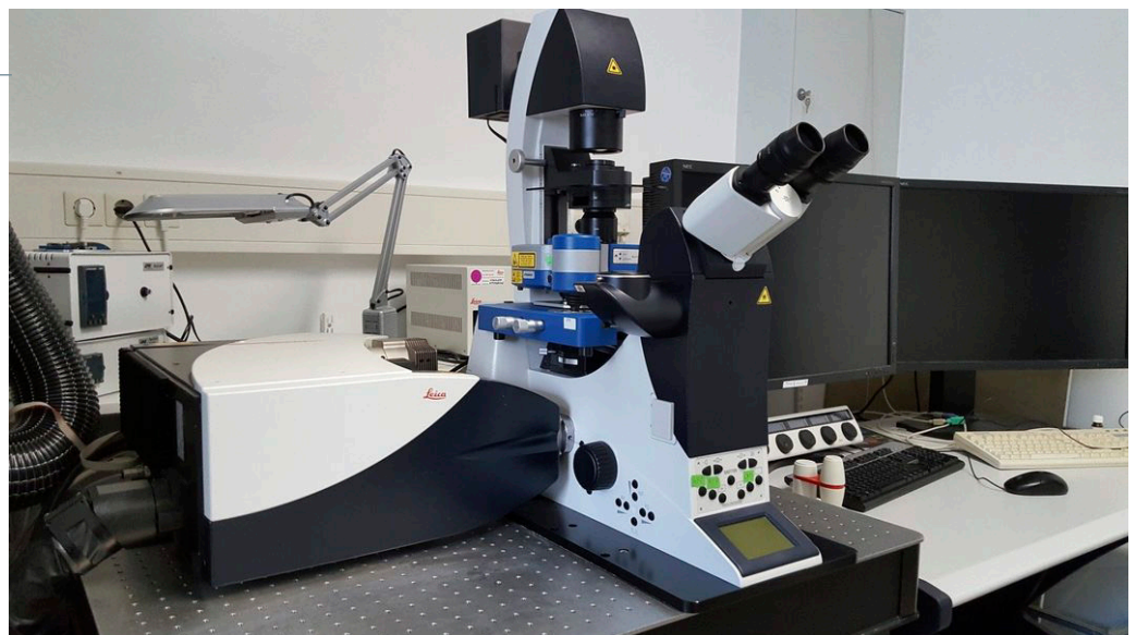
Figure 6: A NanoWizard AFM combined with a Leica TCS SP8 confocal LSM at the Institut für Physiologie II, Münster, Germany. Image courtesy of Prof. Herman Schillers.
