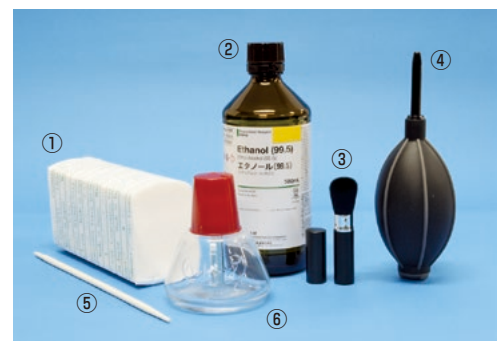
① Lens cleaning paper ② Absolute ethanol ③ Cleaning brush ④ Blower ⑤ Cleaning stick ⑥ Push dispenser
