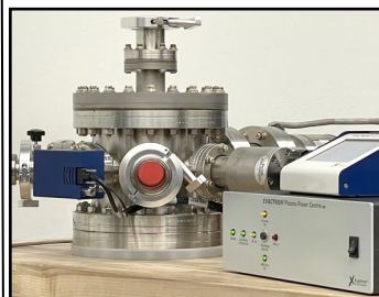
Evactron E16 air plasma and horizontal Power Centre
